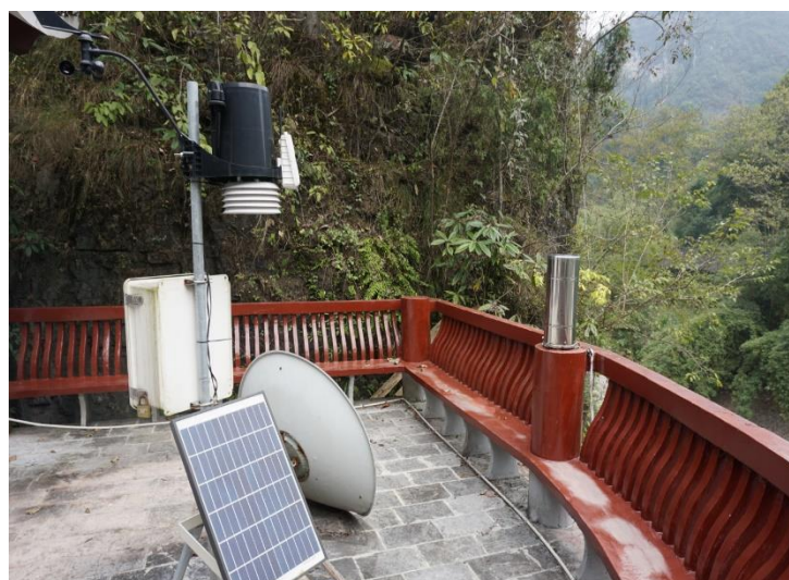
Figure 6 The hydrometeorological monitoring equipment in Shibing Karst
